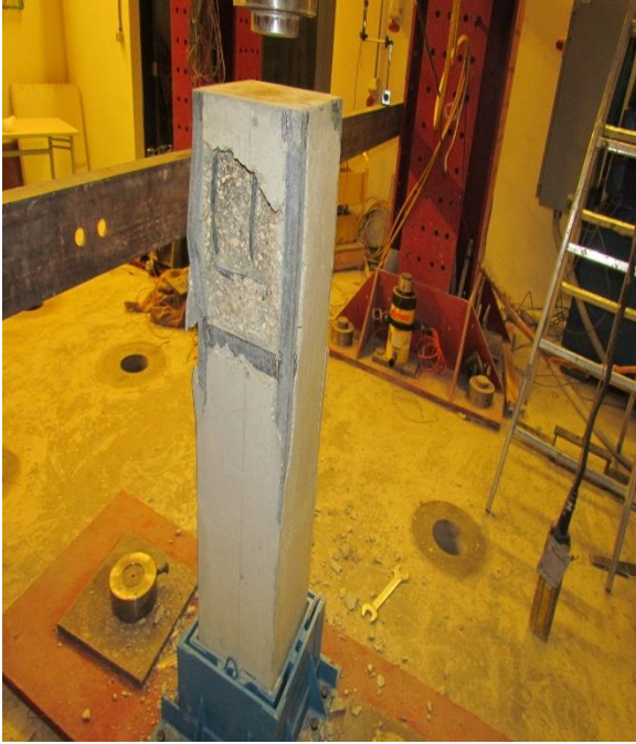
Figure 4-8: Failure of column C31
