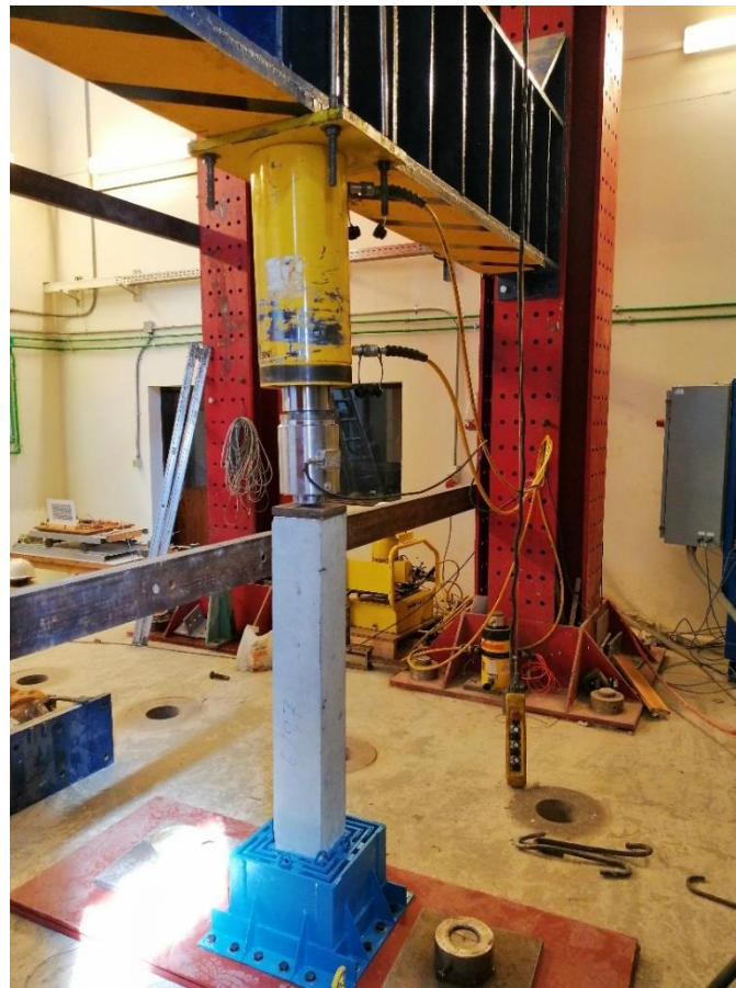
Figure 3-5: Equipment used to test the jacketed columns
