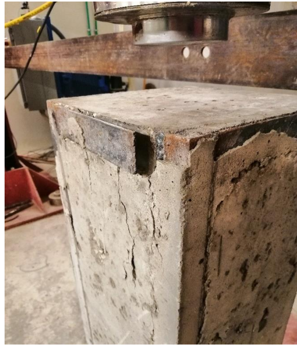
Figure 4-11: Failure of column C42
