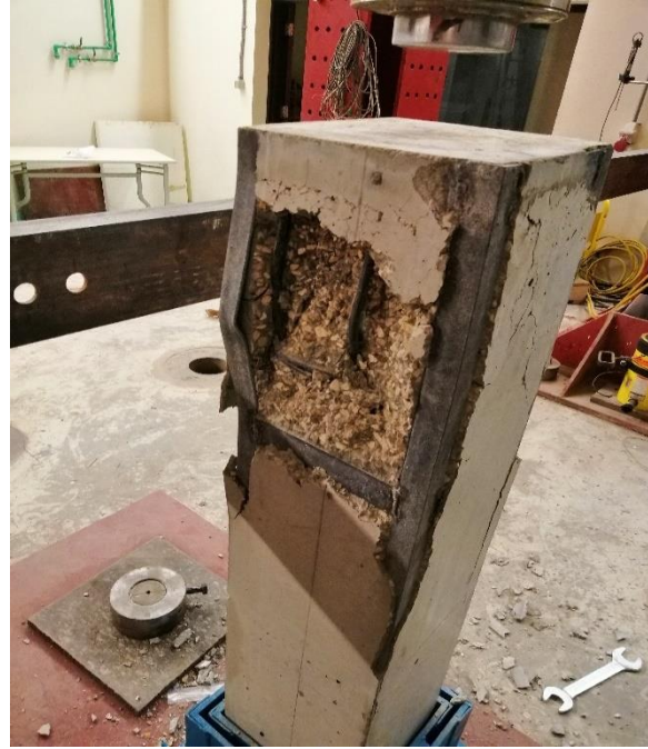
Figure 4-9: Failure of column C32
