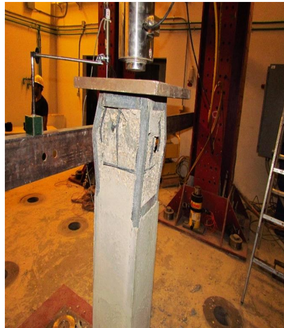
Figure 4-7: Failure of column C22
