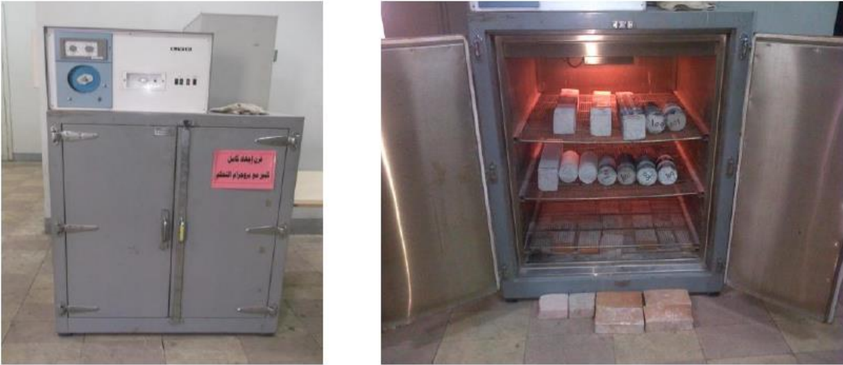
Figure 2-5: Heating the Specimens (Shehab El-Din, 2013)
