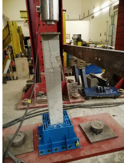
Figure 4-5: Failure of column C12
